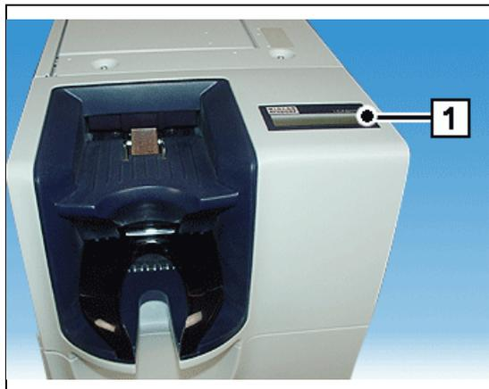
Any malfunctions are signaled to the application by the controller and displayed on the operator display (1).
