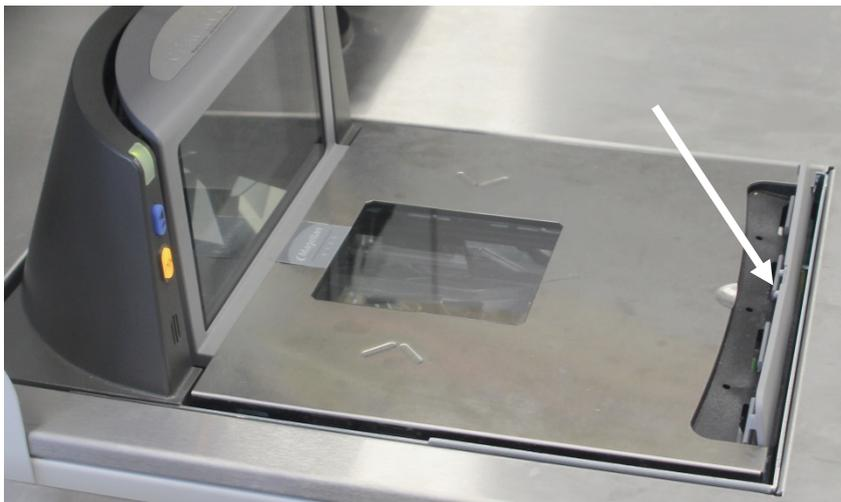
Grasp the lever at the scanner and lift it out of the housing. Take care of the cables.
