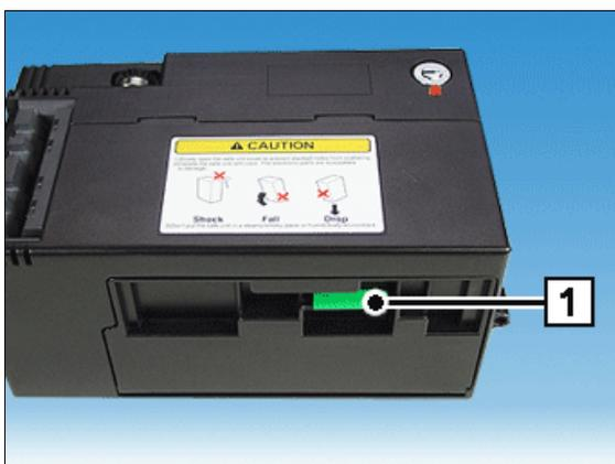
Swing the flap in front of the banknote removal area down by the gripping edge (1).
