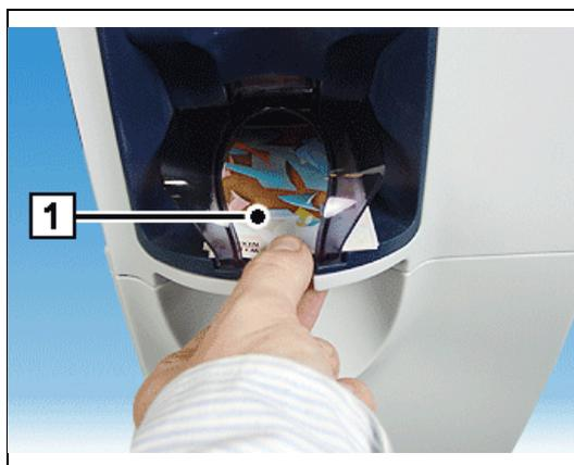
Banknotes totaling the required amount are stored in the reject / output tray (1).
